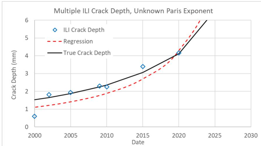
**Figure 6 Analysis of non-linear flaw growth is possible if multiple data sets are available.**
