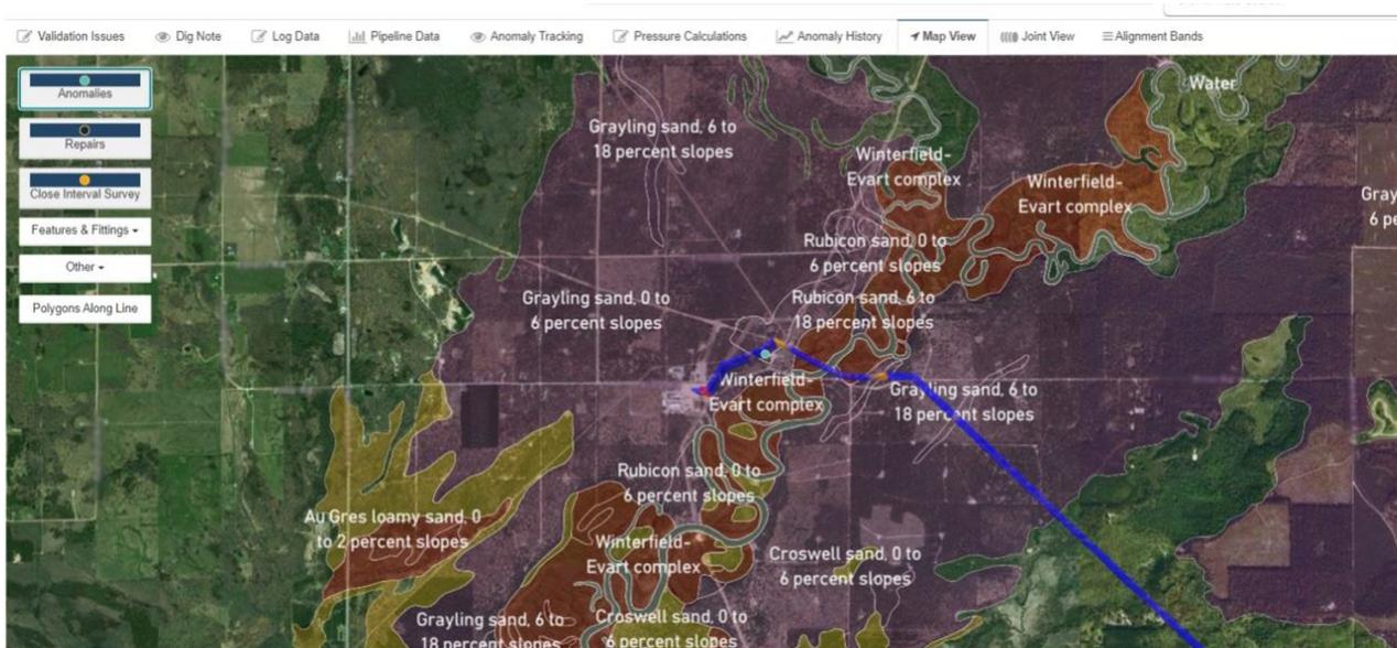
**Figure 10 Soil properties mapping help analysts understand patterns of external corrosion or geohazard threats to their pipelines.**
